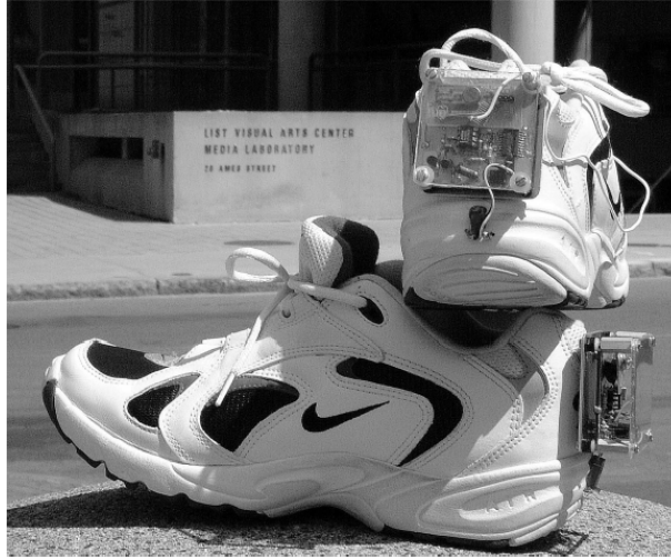
Figure 1.6: Shoe with piezoelectric generation device installed in the heel [8]
